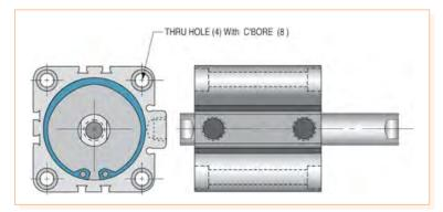
FIGURE 7A. TYPICAL THRU-HOLE MOUNTING
